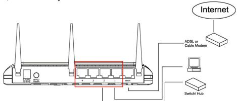
3. Connect the power adapter to the wall socket, and then connect it to the 'Power' socket of the router.
